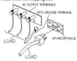
Figure 17. UNV Terminal Lugs (Load)
